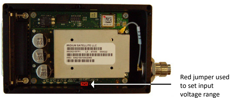
Figure 3: Power Input Setting for the A3LA-RG
