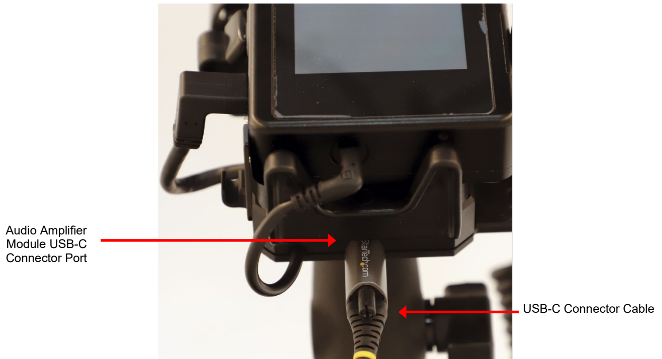
Figure 152: Power Connection to Audio Box
