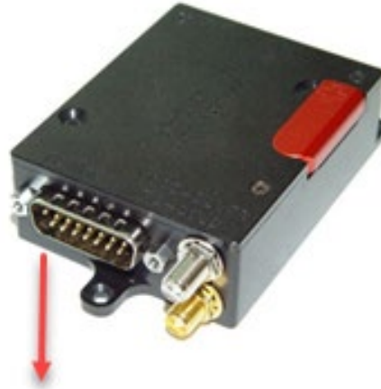
Multi-Interface Connector (Mini DB-15 Connector)
