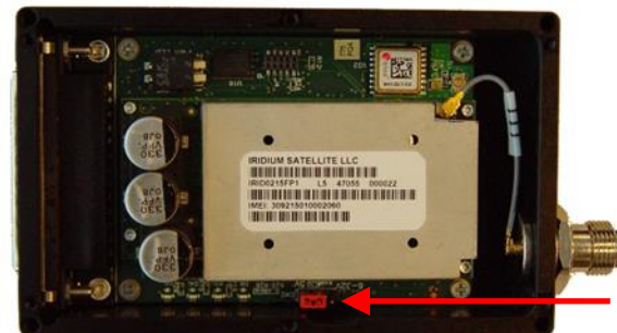
Red jumper used to set input voltage range
