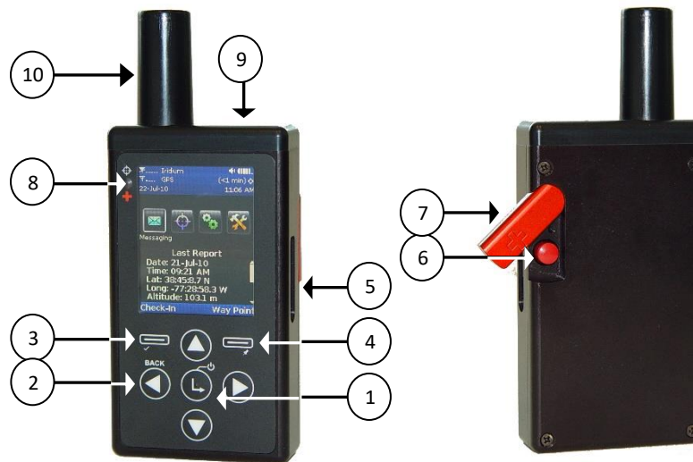
Figure 1: SHOUT nano Buttons, LED, and USB Port
